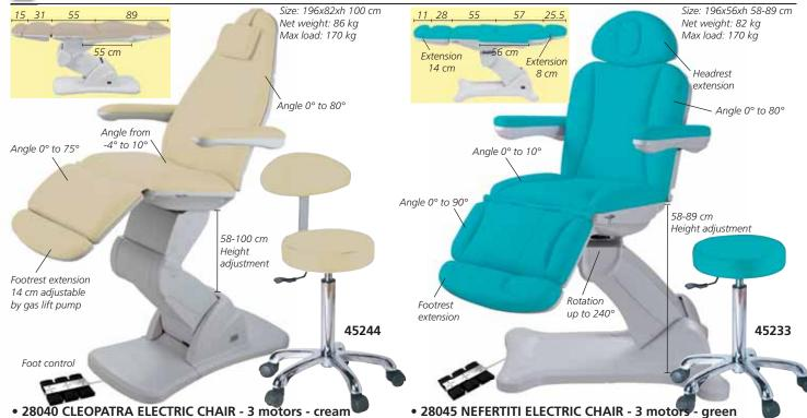
Electrically 3 motors foot crontrolled chair to adjust separately height, backrest and seat inclination. Footrest adjustable by gas lift pump. Reversible arms and adjustable headrest. Operating power: 220-240 V - 50/60 Hz.
